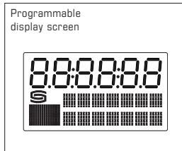
Use the EtherCAT interface to program the **LCD display**.
